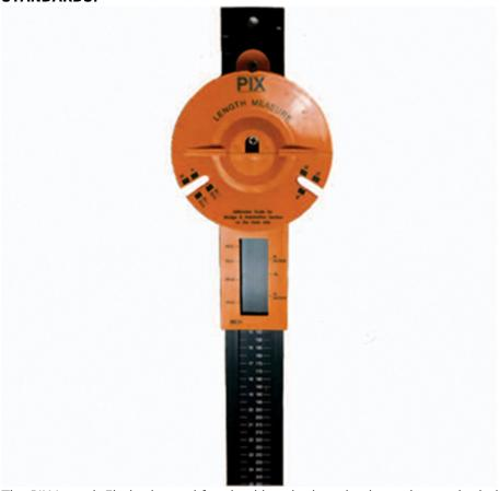
The PIX Length Finder is used for checking the length where size on the belt is not clearly visible. It can aso be used to confirm the type of belt section of the belt. In both caes the results are not exact but very good indicators.
