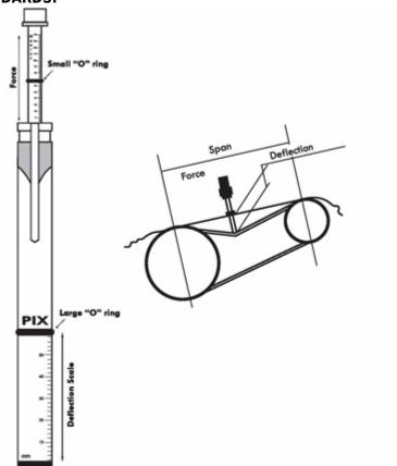
General guidlines for tension measurement of V-belts)
