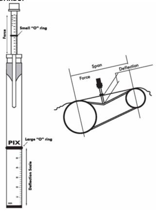
General guidlines for tension measurement of V-belts)
